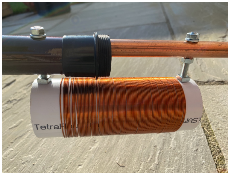
The coil assembly, bolted through the copper pipe and Glass fibre whip.
