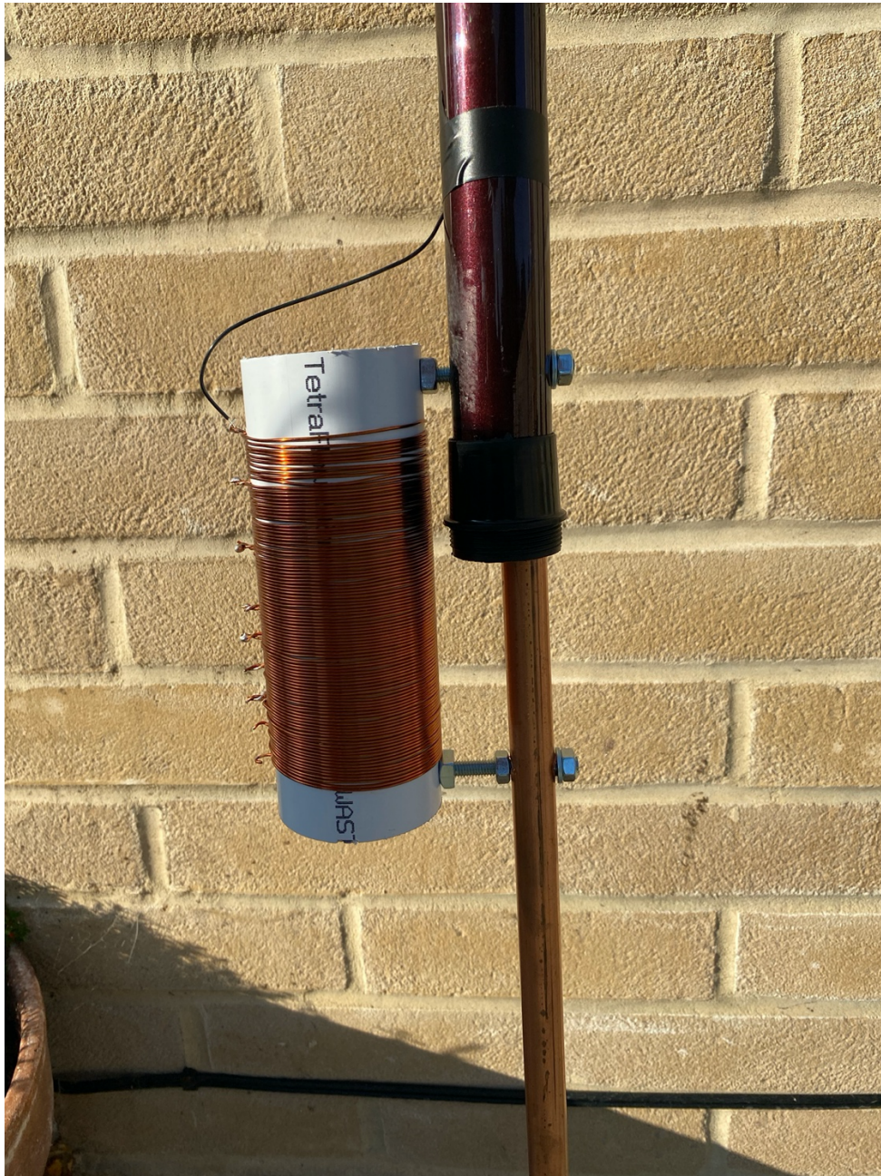
Finished aerial with loading coil.
