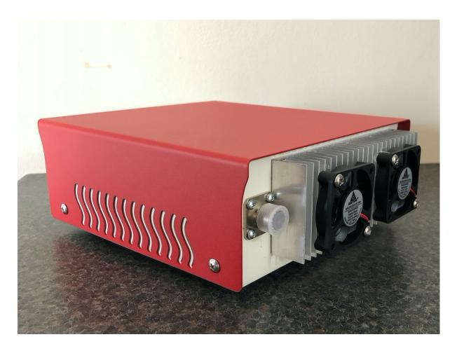
This RF amplifier is designed to operate on the FM Broadcast Band, 88 to 108MHz. The amplifier is wideband, and requires up to 5 Watts drive to give full 100 Watts output. Less input reduces the output, so therefore with 2.5 Watts drive the output level is 50W. It can safely be operated at any output level. The amplifier utilises a Switch Mode Power supply of 24V DC at up to 10 Amps capability.
