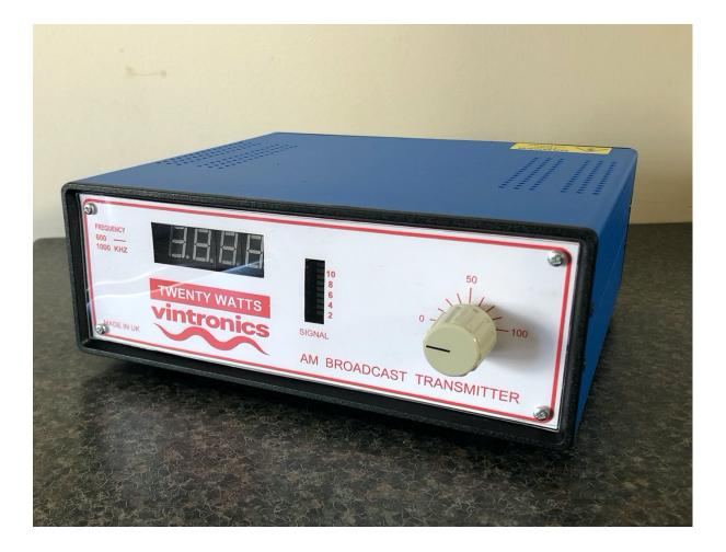
A High-Power version of AM Transmitter, operating between 620KHz and 1024KHz in the Medium Waveband (AM Band) and are designed to be reliable and stable units. They can deliver up to 20 watts of RMS power into a short length aerial. This equates to 80 watts peak power cleanly driven up to 100% modulation.
