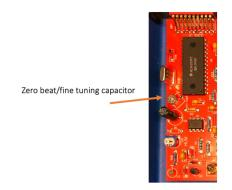
It is possible to fine-tune the operating frequency by adjusting VC1 on the main circuit board. (see pic) This adjustment is for 'zero-beat' of the signal (in comparison to another signal\*) but is not an essential adjustment and can be left if not required. (cap may look different)
