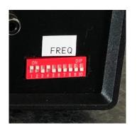
On the rear of the unit, the DIP switches determine the frequency. (in this case up is 'on' and down is 'off')
