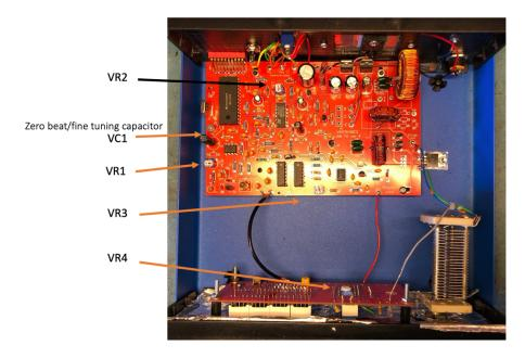
The Variable Inductor is located to the top-right of the circuit board. (the round coil)
