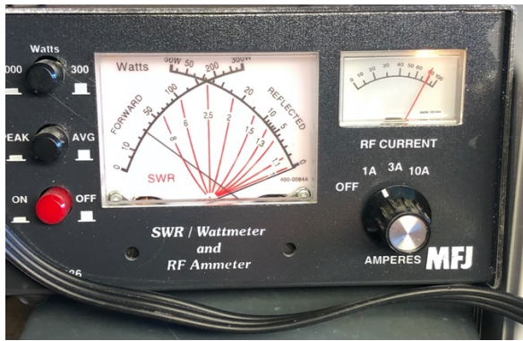
30W at 1602KHz into 50 Ohm load.
