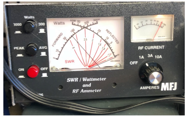
80W peak shown at 1602KHz into 50 Ohm load.
